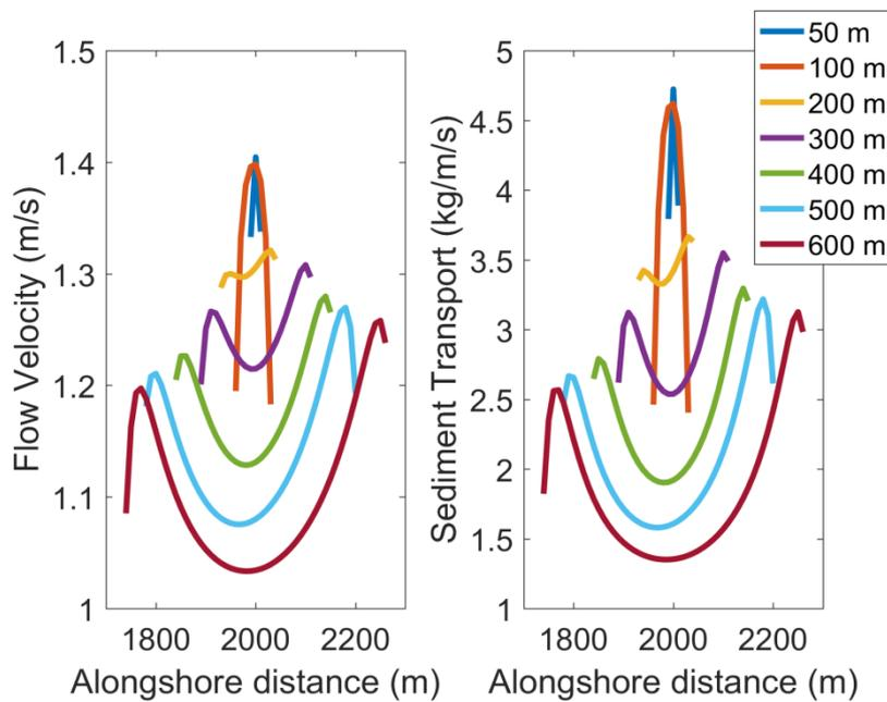
Figure 5. a) Flow velocity and b) Sediment transport along the washover opening for different washover widths for a washover height of 2.0 m.
