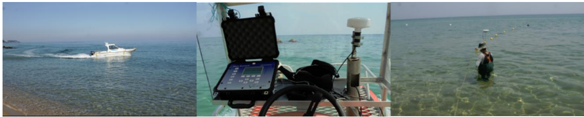
Figure 3. Survey procedure for beach topography and bottom bathymetry; a survey vessel (left), single-beam echo sounder and GPS (middle), and RTK-GPS (right).
