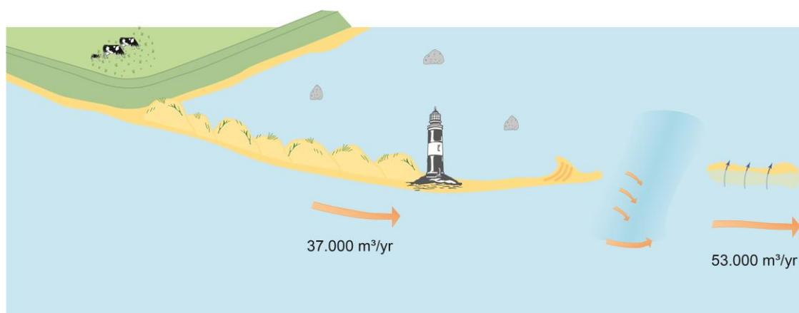
Figure 6. Conceptual model of the barrier morphodynamics at Rødsand.
