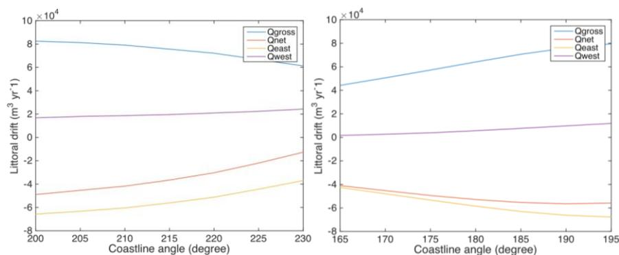
Figure 4. Q-alpha curves from the LITDRIFT model.
