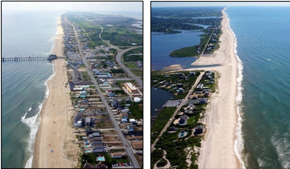
Figure 4. Oblique aerial photos showing the rhythmic topography of both project sites after nourishment, a similar feature to the pre-nourishment condition indicating beach fill equilibration in the longshore direction. [LEFT] Photo taken on 28 June 2015 at Nags Head looking southwest. [RIGHT] Photo taken on 30 June 2016 at Bridgehampton looking east.
