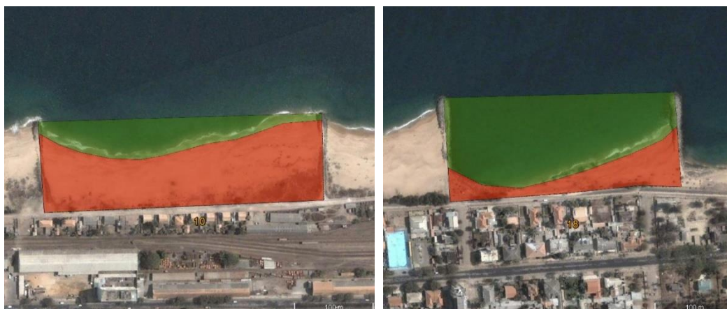
Figure 4. The groyne fill ratio is defined as the plan form area of dry beach relative to the total area between two neighbouring groyne. Left: Groyne compartment 10. Right: Groyne compartment 18. Both from 2004-07-28.
