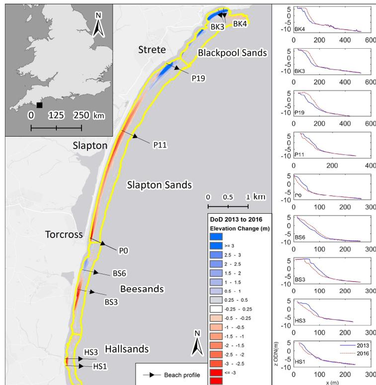
Figure 3. Left: Digital elevation model of difference (DoD) of Start Bay from 2013 to 2016 (Wiggins, in prep), including subaerial and subtidal extents. Right: Subaerial to subtidal profiles extracted from digital elevation models, from 2013 (blue) and 2016 (red)
