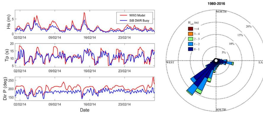
Figure 6. Left: from top to bottom; Significant wave height (Hs), peak period (Tp), peak direction (Dir P) for WaveWatch III Modelled wave data (red), and measured wave buoy data (blue) for the month of February 2014. Right panel: WaveWatch III model node wave rose for the years 1980 – 2016
