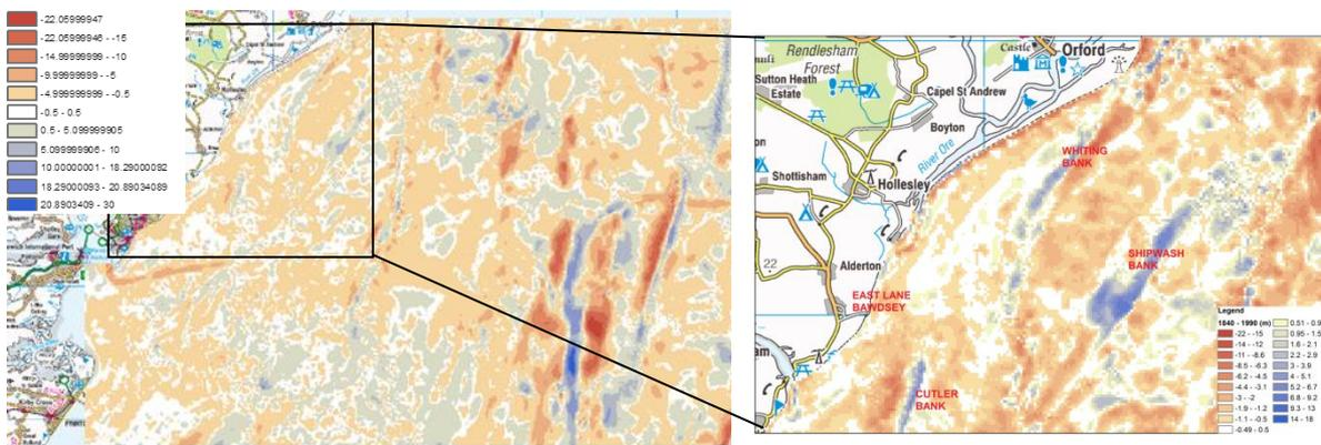
Figure 4. Bathymetric changes near study frontage (1840-1990) (Data source: UCL)
