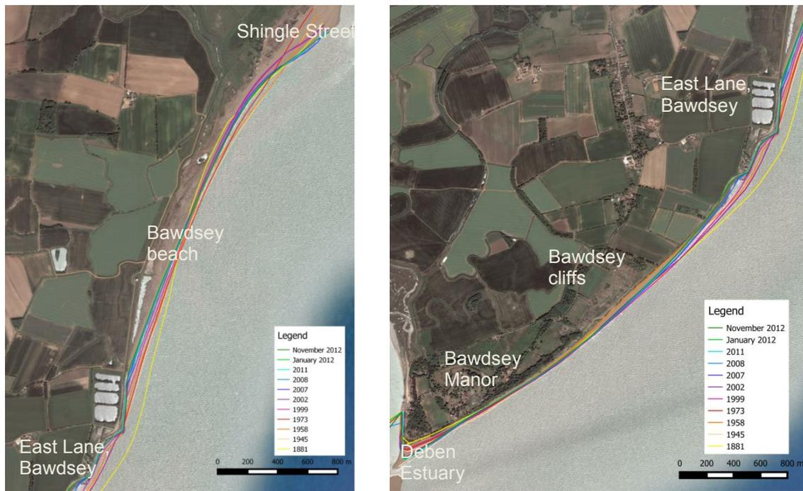
Figure 2. Historical shoreline positions – left pane: Shingle Street to East Lane, right pane: East Lane, Bawdsey to River Deben (Data from Burningham and French, 2017).
