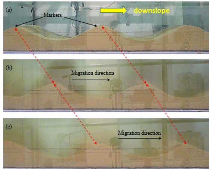
Figure 11 Ripple migration on sloping bottom (test TB02,  $U_{bm}=0.75\text{m/s}$ ,  $T=6.25\text{s}$ ,  $\eta=82\text{mm}$ ,  $\lambda=541\text{mm}$ , slope  $\beta=2.6^\circ$ ). The time interval between two successive frames is 190 wave periods.
