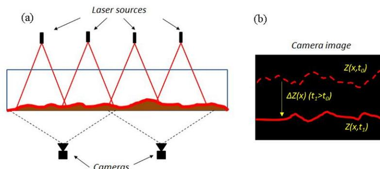
Figure 2 the general concept of the LBP system: (a) system setup, (b) image of laser line on the moveable bed
