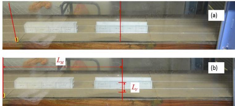
Figure 4 Image rectification based on the calibration image: (a) raw image, (b) rectified image
