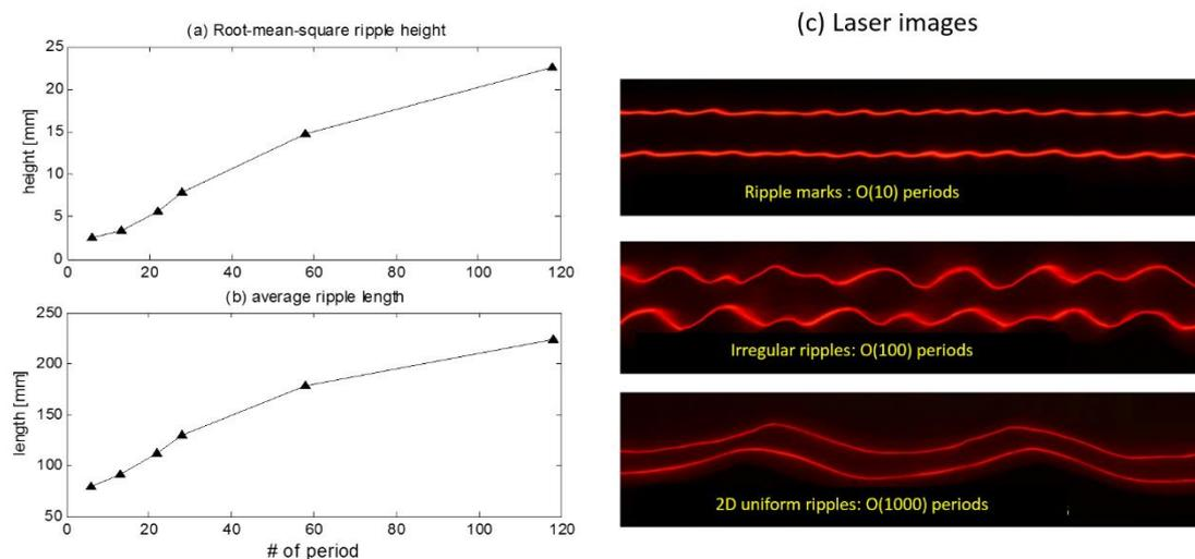
Figure 9 history of ripple development from a flat sand bottom: (a) variation of root-mean-square ripple height for test TC, (b) variation of average ripple length for test TC, (c) typical laser images showing the change of bottom profile.
