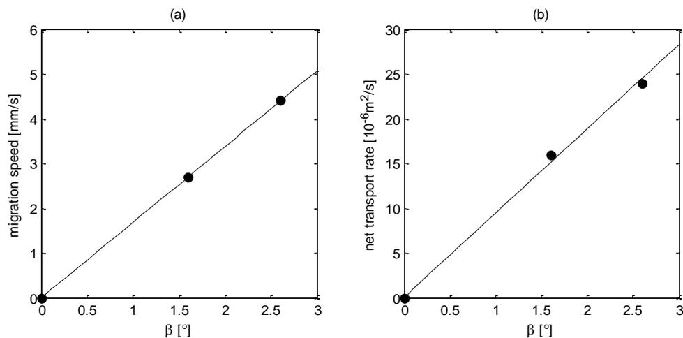
Figure 12 Migration speed and net sediment transport rate for test TB01 and TB02.
