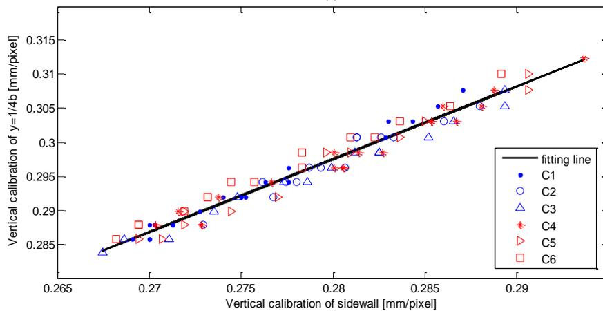
Figure 6 Empirical formula for correlating the vertical calibration parameter of a laser line (the one closer to the camera) with that of the front sidewall (C1 to C6 indicates six cameras)
