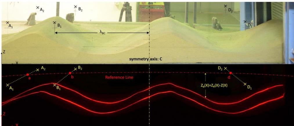
Figure 7 Determination of the reference line for calculating bottom profile
