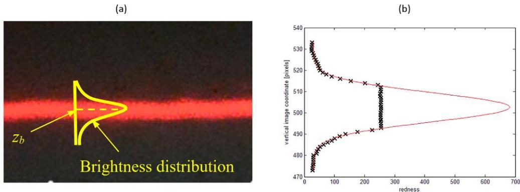
Figure 5 Locating the movable bottom on the laser-line image (a) laser-line image (b) fitted normal distribution (crosses are measured redness values, solid line is the fitting)
