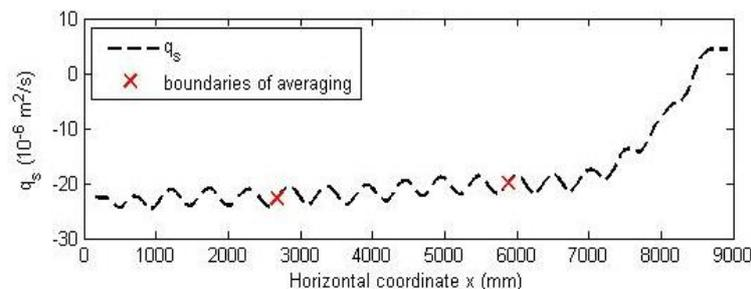
Figure 13 net sediment transport rate for test TB02
