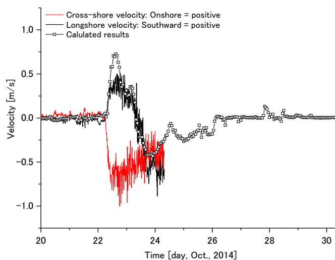
Figure 11. Observed and calculated results of current velocities at  $x = 245$  m.
