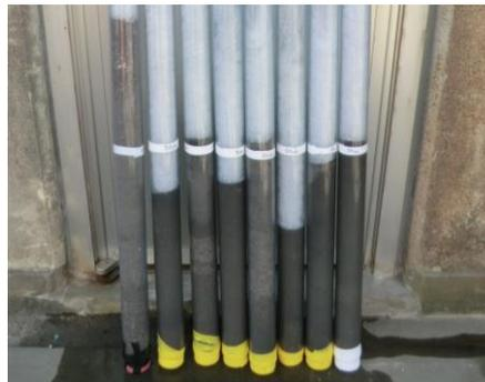
Picture 2. Collected vertical core samples.
