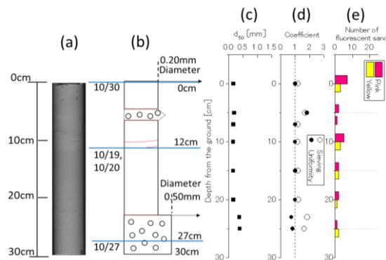
Figure 8. Vertical distributions of the sand core collected at  $x = 215$  m. (a) X-ray CT picture (b) stratigraphic column, (c) median diameter, (d) sieving and uniformity coefficients, and (e) number of fluorescent sand tracers.
