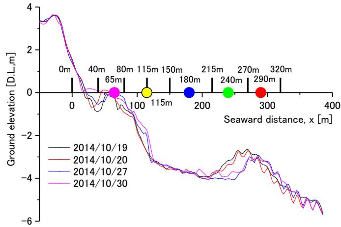
Figure 2. Seabed profile changes during the experiments.
