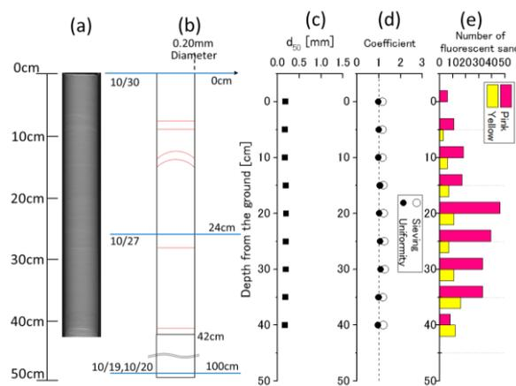
Figure 6. Vertical distributions of the sand core collected at  $x = 115\text{ m}$ . (a) X-ray CT picture (b) stratigraphic column, (c) median diameter, (d) sieving and uniformity coefficients, and (e) number of fluorescent sand tracers.
