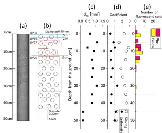
Figure 7. Vertical distributions of the sand core collected at  $x = 150\text{ m}$ . (a) X-ray CT picture (b) stratigraphic column, (c) median diameter, (d) sieving and uniformity coefficients, and (e) number of fluorescent sand tracer.
