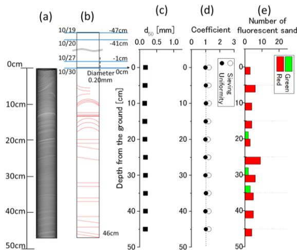
Figure 9. Vertical distributions of the sand core collected at  $x = 270$  m. (a) X-ray CT picture (b) stratigraphic column, (c) median diameter, (d) sieving and uniformity coefficients, and (e) number of fluorescent sand tracers.
