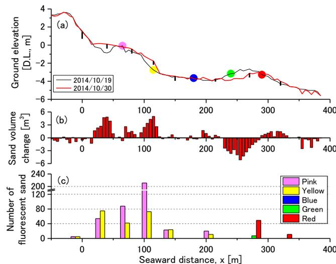
Figure 10. (a) Beach profile change, (b) sediment volume difference during the experiment, and (c) spatial distribution of the number of fluorescent sand tracers.
