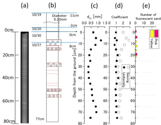
Figure 4. Vertical distributions of the sand core collected at  $x = 0$  m. (a) X-ray CT picture (b) stratigraphic column, (c) median diameter, (d) sieving and uniformity coefficients, and (e) the number of fluorescent sand tracers.
