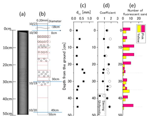
Figure 5. Vertical distributions of the sand core collected at  $x = 80$  m. (a) X-ray CT picture (b) stratigraphic column, (c) median diameter, (d) sieving and uniformity coefficients, and (e) number of fluorescent sand tracers.
