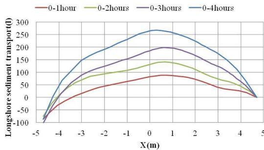
Figure 9. Total amount of sand transported alongshore.
