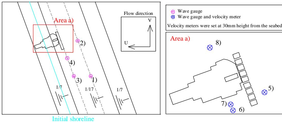
Figure 15. Locations of wave gauges and velocity meters.
