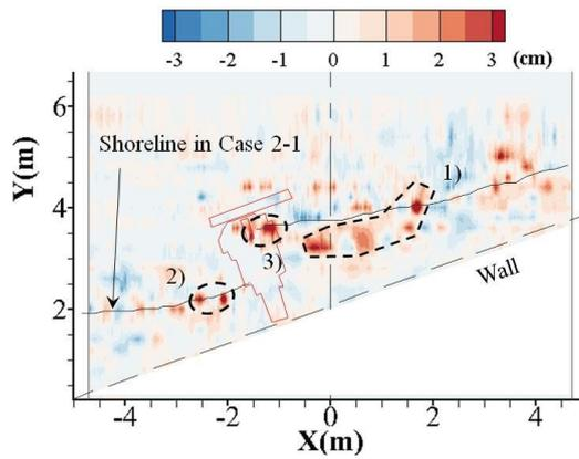
Figure 18. Difference in bathymetry between Cases 1-1 and 2-1.
