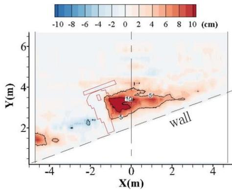
Figure 12. Bathymetry change in Case 1-1.
