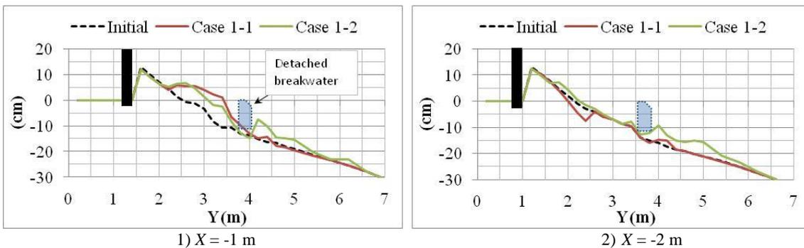
Figure 14. Cross-section of bathymetric change.
