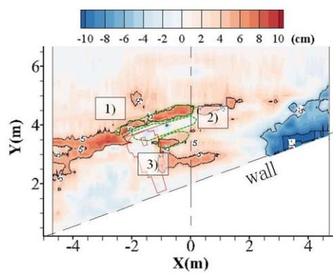
Figure 13. Bathymetry change in Case 1-2.
