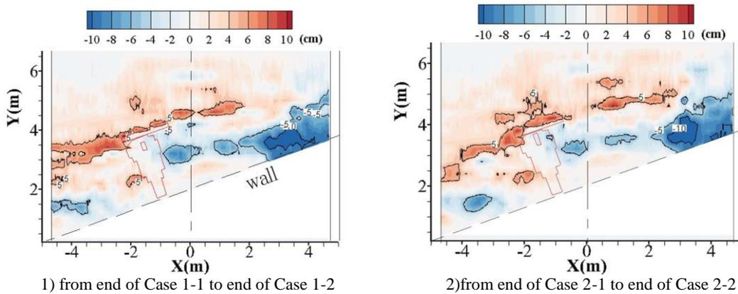
Figure 19. Bathymetry change after 2 hours of storm waves.
