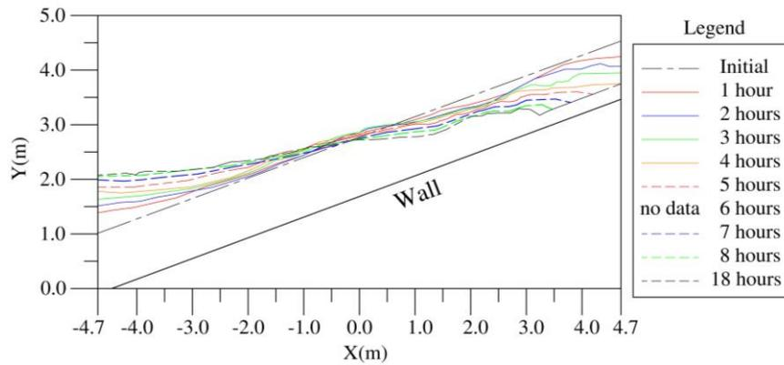
Figure 8. Shoreline change in pre-experiment without structures.
