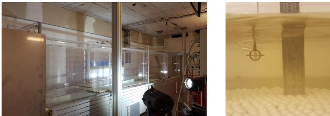
Figure1. Left The flume of the IPR (Institute of Physics of Rennes); Right the velocity probe on the rough bed.
