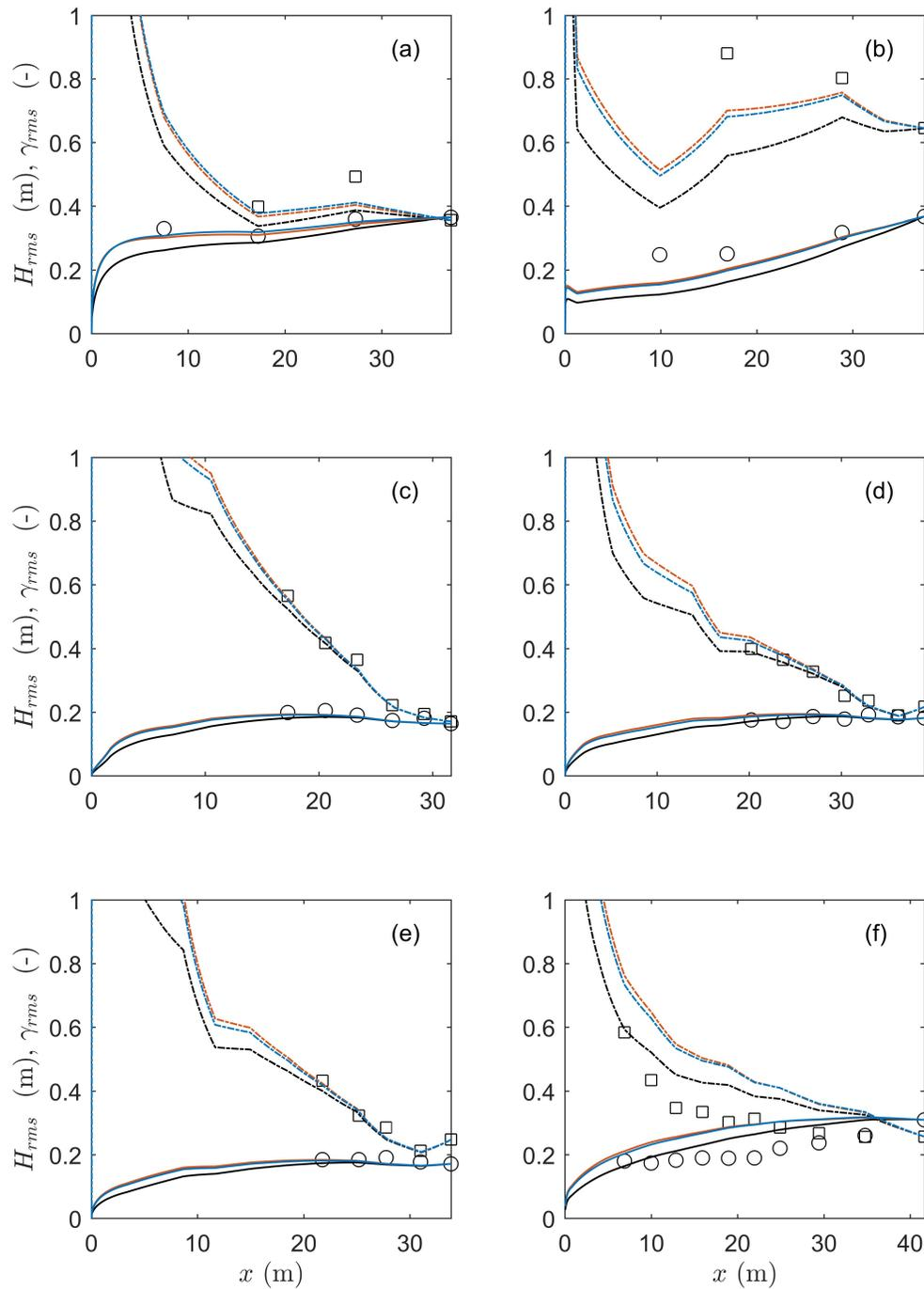
Figure 5. Comparison of measured data on wave heights (open circles) and  $\gamma$  values open squares) with the cross-shore wave height transformation model predictions of wave heights (solid lines) and  $\gamma$  values (dashed lines) for six data runs (see Table 1 for details). Each panel shows model results from models with three different wave height distributions:
