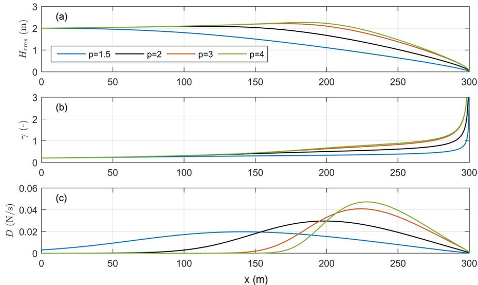
Figure 3. The effect of varying the value of  $p$  on (a) cross shore wave height transformation ( $H_{rms}$ ), (b) gamma values ( $\gamma$ ), and (c) energy dissipation ( $D$ ) for a plane beach profile with  $\tan\beta = 1/30$  for four different values of  $p$ :  $p = 1.5$  (blue line),  $p = 2$  (black line),  $p = 3$  (red line), and  $p = 4$  (green line). The model was run with initial conditions of  $H_{rms} = 2$  m,  $T = 8$  s, and  $h(x = 0 \text{ m}) = 10$  m.
