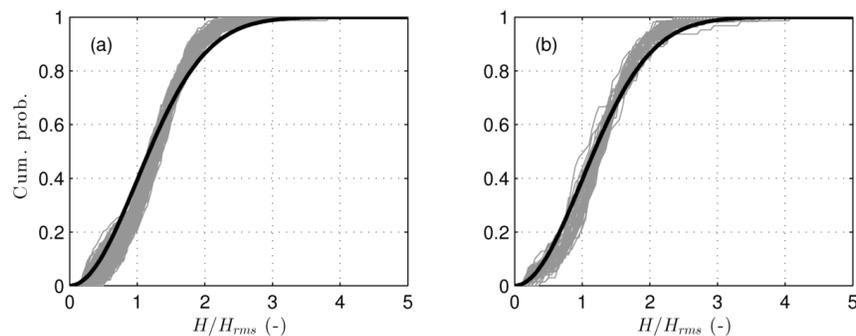
Figure 2. Cumulative probability distribution of normalised wave height,  $H/H_{rms}$ , for each data run (grey lines) compared to the cumulative Rayleigh distribution function (black line) for two example deployments: (a) Moreton Island 8 December 2008, and (b) The Spit, Gold Coast, 12 March 2009 (from Power *et al.*, 2016).
