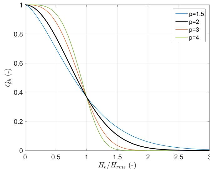
Figure 3. The effect of varying the value of  $p$  on the fraction of broken waves ( $Q_b$ ) for four different values of  $p$ :  $p = 1.5$  (blue line),  $p = 2$  (black line),  $p = 3$  (red line), and  $p = 4$  (green line).
