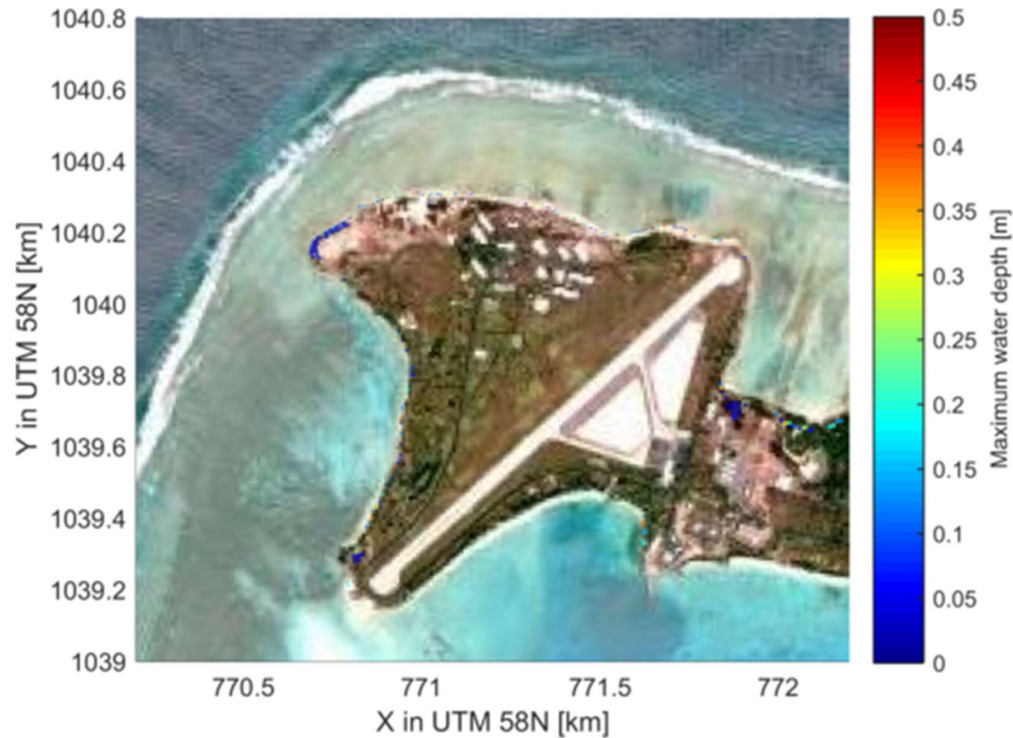
Figure 4 Modeled inundation depth for the calibrated 2D model during the March 2014 overwash event on Roi-Namur. The color bar denotes the maximum water depth on the island during the March 2014 overwash event.
