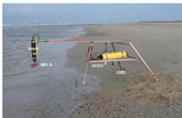
Figure 3. The tripod with the installed instruments at low tide on September 30, 2012
