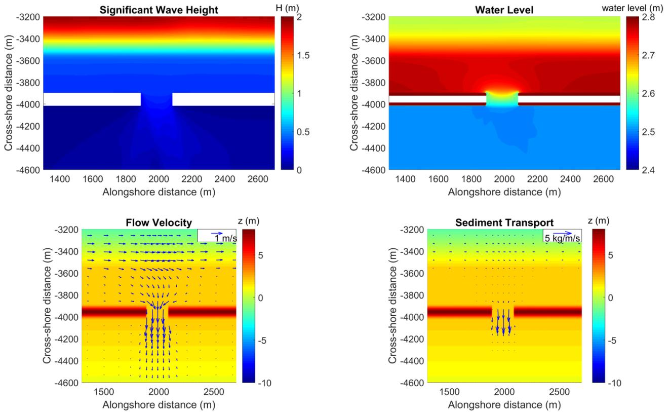
Figure 4. The hourly averaged a) Significant short wave height and b) Water level. Vector plots of c) the flow velocity and d) the sediment transport.
