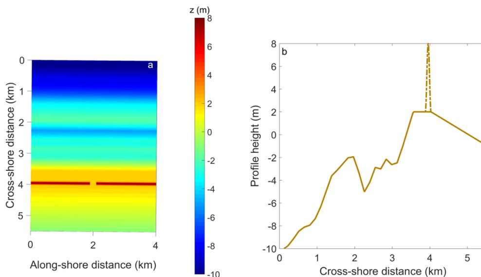
Figure 3. a) The reference profile in a) 2D and b) 1D. The washover height is 2.0 m, the washover width 200 m, the beach berm width 300 m and the foreshore slope 0.01 m/m.
