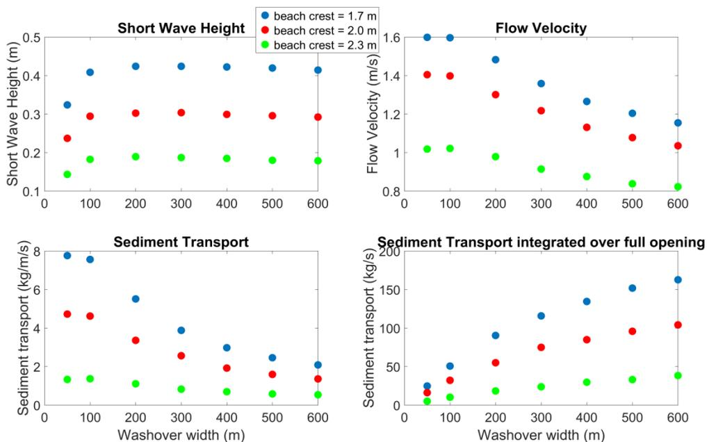
Figure 6. Parameters in the middle of washover opening for several combinations of washover width and height. a) Significant short wave height. b) Flow velocity. c) Cross-shore sediment transport. d) Cross-shore sediment transport integrated over the entire opening.
