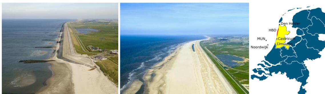
Figure 2: Hondsbosse and Pettemer Zeewering, a sandy coastal flood protection near Petten, the Netherlands. The original, hard protection in 2005 (left) and the new sandy coastal protection in 2015 (right).
