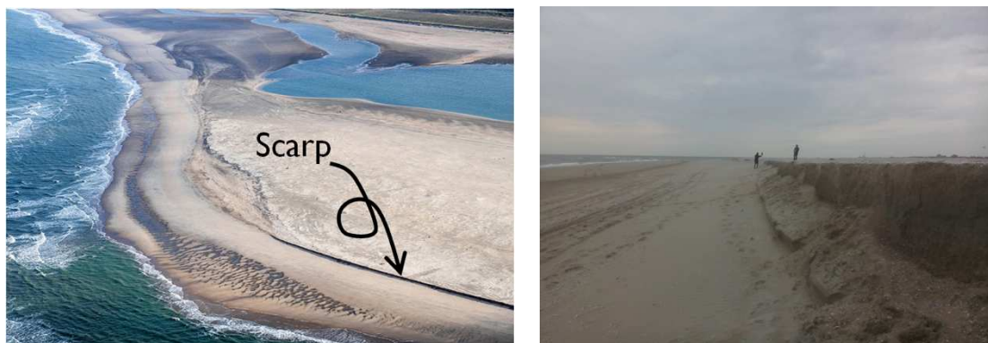
Figure 1. Beach scarps along the perimeter of the Sand Engine mega-nourishment (11 November 2015), the Netherlands. Aerial image: Rijkswaterstaat/Joop van Houdt.
