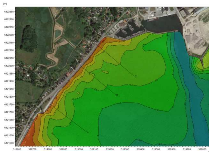
Figure 1. Satellite picture of study area with existing bathymetry map showing location of three beach profiles used to plan the nourishment scheme.
