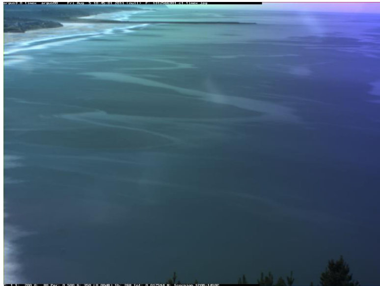
Figure 2. Example one-minute wave-averaged image from Agate Beach, Oregon. Slicks are revealed once the clutter of ocean waves are removed. By display these images in sequence (every minute), the movement of these features is revealed.
