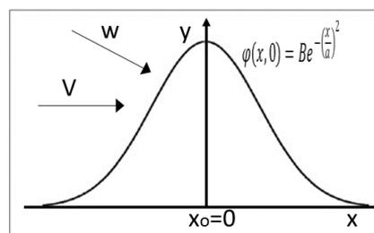
Figure 6. Schematic representation of a bell-curved mega-nourishment at  $t=0$ . It is exposed to a longshore sea current with velocity  $V$  and a constant wave event  $w$ .
