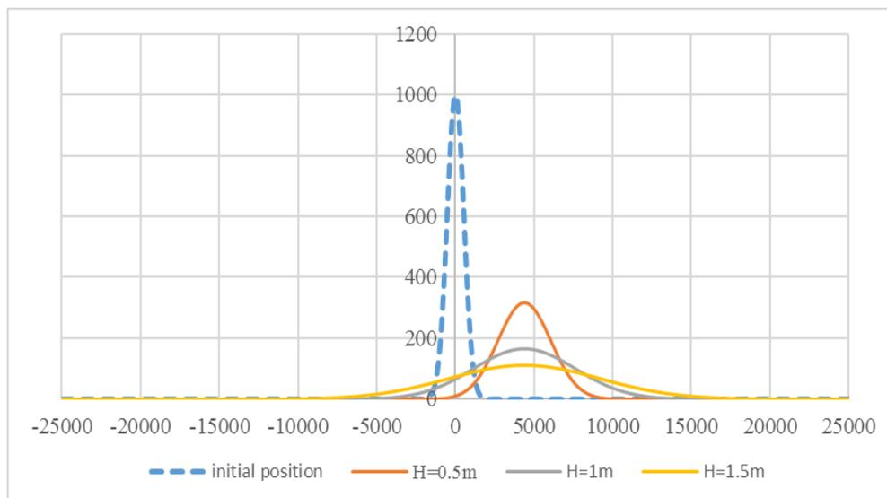
Figure 9. The 10-year morphodynamic evolution of a mega-nourishment for different values of the diffusion coefficient  $\epsilon$ , corresponding to wave height  $H=0; 0.5m; 1m; 1.5m$ . The velocity of the longshore current remains constant and equal to  $0.5 m/hr$ .
