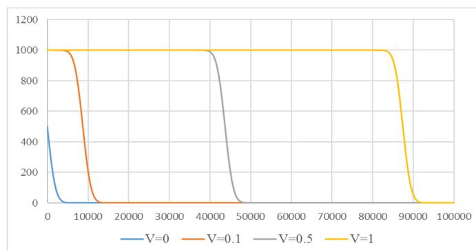
Figure 7. The ten-year morphodynamic evolution of the mega-nourishment for different values of the velocity of the longshore current:  $V = 0; 0.1; 0.5$ ; and 1 m/hr. and constant wave event ( $H = 0.5$  m and  $T = 6$  sec).
