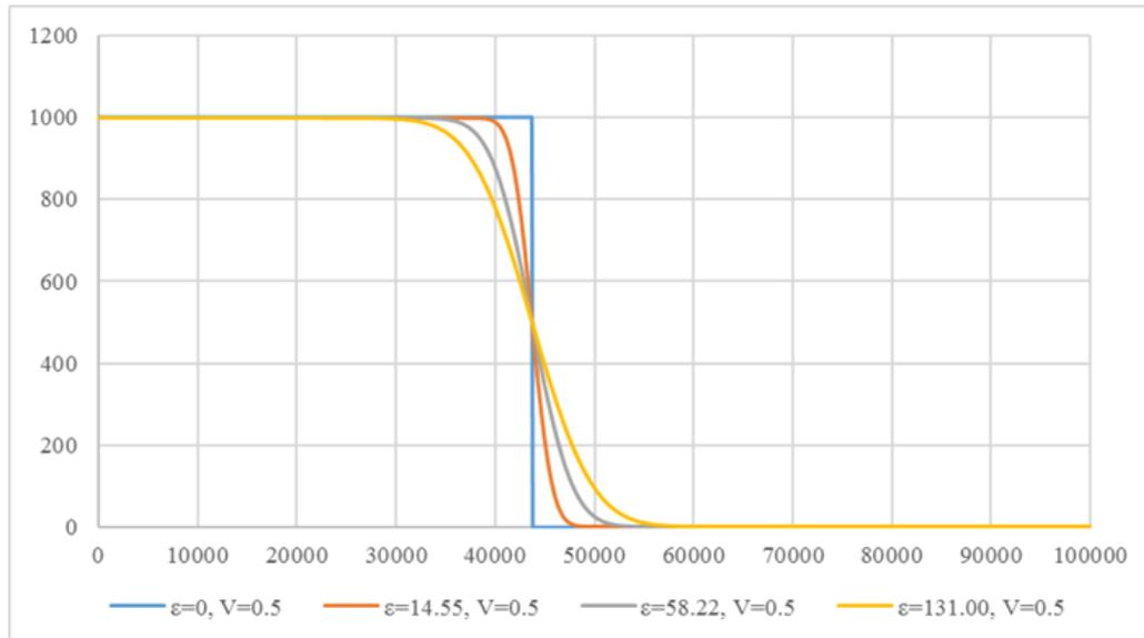
Figure 8. The 10-year morphodynamic evolution of a mega-nourishment for different values of the diffusion coefficient  $\epsilon$ , corresponding to wave height  $H=0; 0.5m; 1m$ ; and  $1.5m$ , and constant wave period  $T=6 sec$ . The longshore current is considered constant in time with  $V=0.5 m/hr$ .
