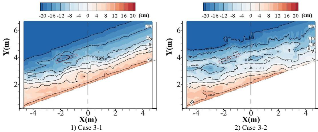
Figure 21. Bathymetry in Cases 3-1 and 3-2 (elevation from water level)
